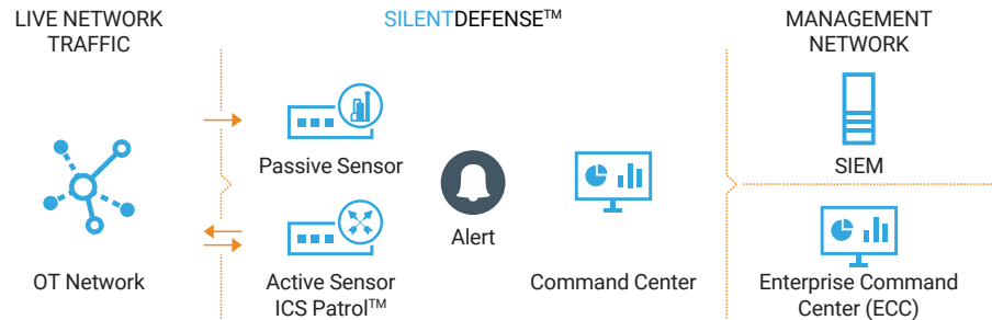
Basic SilentDefense and ICS Patrol Deployment Model
