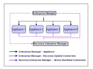
This connection is used to manage network Appliances when the recovery Enterprise Manager is switched over as the primary Enterprise Manager. Communication between the Enterprise Manager and the Recovery Enterprise Manager is performed on port 13000/TCP using standard TLS encryption. You may set up one Recovery Enterprise Manager in your enterprise.
