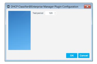
**5.** Select the **Test** button. A confirmation popup opens. For the duration of the test (as configured in step 4), the plugin listens for DHCP requests on the device.
