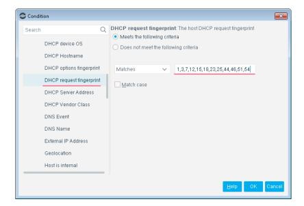
2. The new condition matches the DHCP request fingerprint of the printer.
