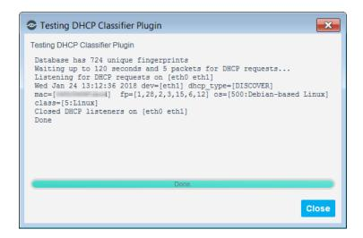
**6.** Trigger the DHCP request from an endpoint with a known MAC address within the managed network segment.
