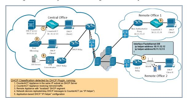
The figure above shows the following typical routing paths for DHCP traffic:
