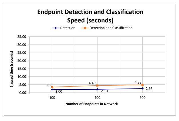
The above data points reflect the best speeds observed for each network size tested for multiple iterations. An unprecedented detection rate in the NAC industry was recorded for 500 devices in less than 5 seconds, proving scalability. There is a correlation between the number of endpoints and speed of detection and classification, although the increase is not necessarily linear.
