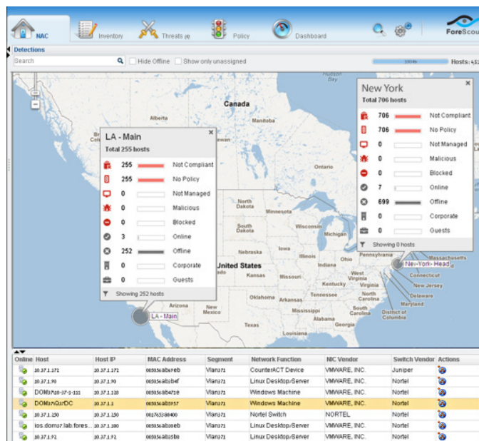
Figure 1: ForeScout CounterACT provides both high-level and detailed information about devices on your network.
