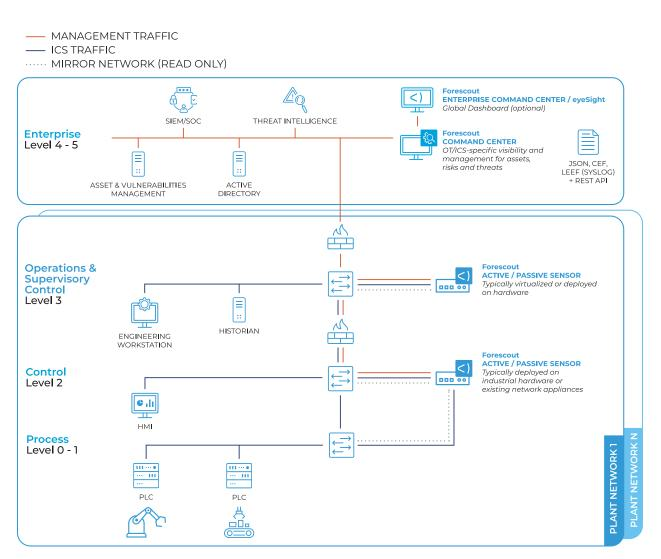
Figure 1: Typical deployment architecture for manufacturing environments combines passive network monitoring with active discovery and integrations to automate cyber security across the OT/ICS environment and beyond.
